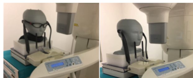
Figure 1: Set up of 30 year old female phantom in proper scanning position in the Carestream Kodak 9000 3D CBCT unit.
